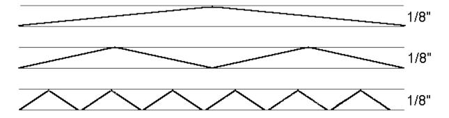
Since all these floor profiles would meet the 1/8th" spec, the straightedge specs themselves simply were not capable of controlling the floor profile.
