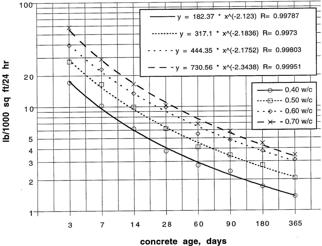
Data from H. W. Brewer, "Moisture Migration-Concrete Slab-on-Ground Construction" Jnl PCA R&D Labs, vol 7, no 2,1965. (4" slabs, dried one side at 73F/50%RH, moisture vapor other side)
